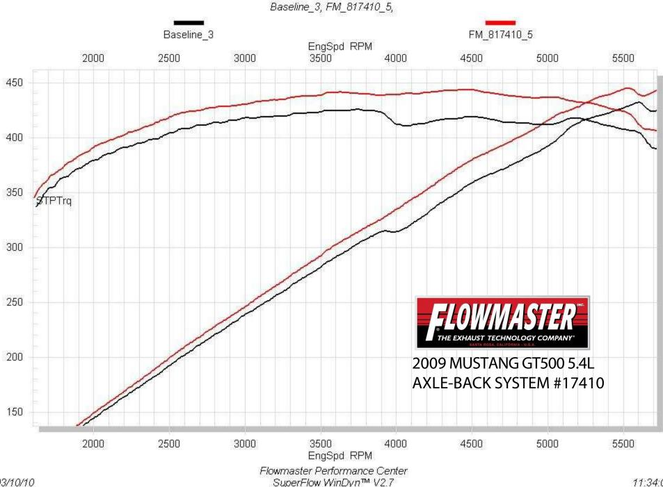
STP Corrected Wheel Power vs. RPM
