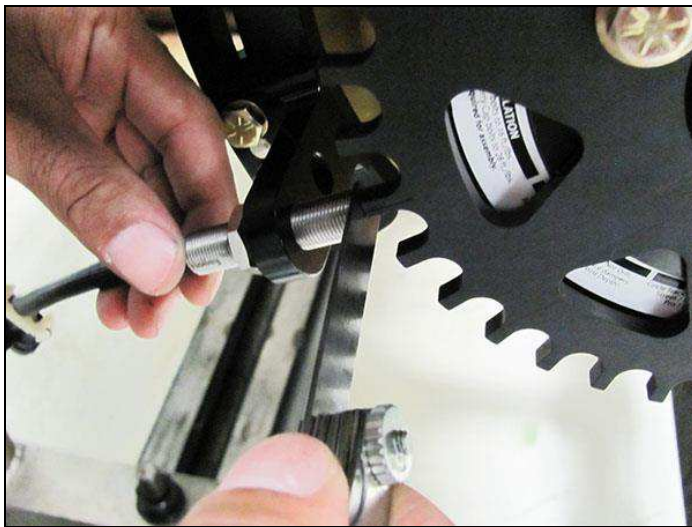
Figure 8: Adjusting the Sensor Gap
