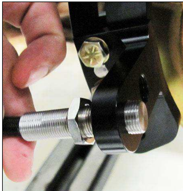
Figure 3: Installing the Sensor.
