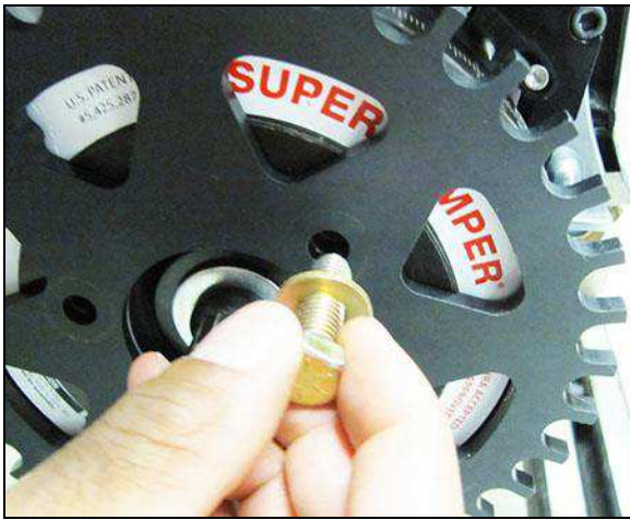
Figure 7: Fastening the Crank Wheel to the Balancer
