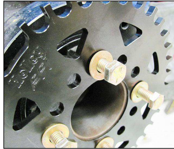
Figure 7: Fastening the Crank Wheel to the Balancer
