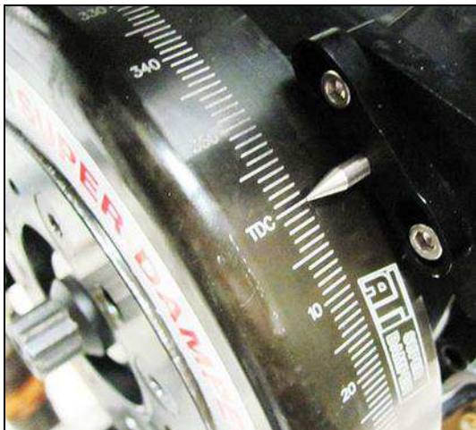
Figure 5: Rotating the Engine to TDC #1
