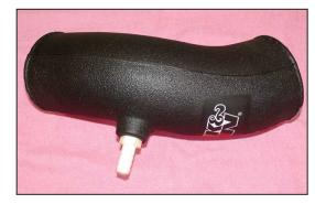
12. Install the provided 1/4" npt fitting into the intake tube as shown.
