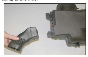
14. Remove the factory fresh air hose from the air box as shown.
