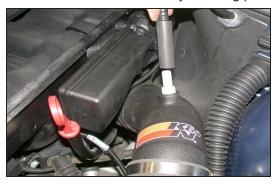
29. Using the supplied silicone hose, attach the factory vent hose to the npt fitting on the intake tube.
