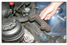
11. Unstrap the heater hose from the lower air box locator, and then pull up to remove the lower air box locator from the vehicle.
