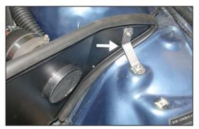
26. Install the provided bracket onto the heat shield and inner fender with the provided hardware as shown.
