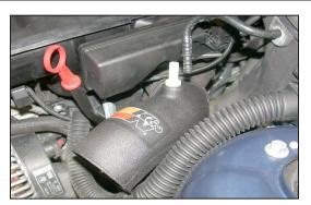
13. Install the K&N<sup>®</sup> intake tube into the factory lower intake hose and secure with the factory hose clamp.
