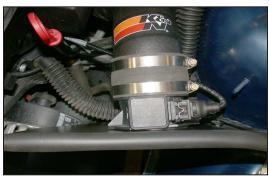
30. Reconnect the mass air sensor electrical connection.
