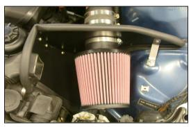
31. Install the air filter and secure with the hose clamp provided.
