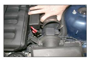
5. Loosen the hose clamp that secures the intake tube to the mass air sensor and then disconnect the intake tube from the mass air sensor as shown.
