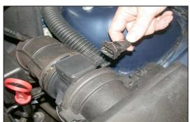
2. Depress the wire-locking clip and disconnect the mass air sensor electrical connection.
