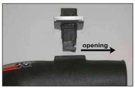
19. Install the mass air sensor assembly into the  $K\&N^{\text{@}}$  intake tube.
