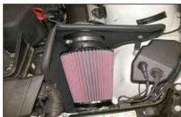
24. Install the K&N $^{\circ}$  air filter onto the K&N $^{\circ}$  intake tube and secure with the provided hose clamp.
