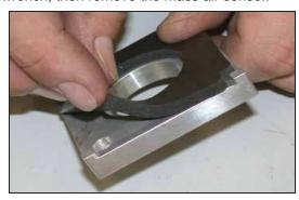
17. Install the provided gasket onto the mass air adapter as shown, sticky side down.
