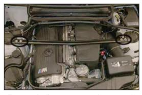
2. Remove the four 13mm nuts that secure the strut tower brace to the vehicle, then remove the brace from the vehicle.
