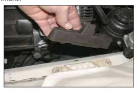
8. Lift up on lower air box mount and then remove from vehicle.
