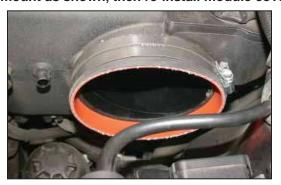
15. Install the silicone hose (08612) onto the intake plunem as shown using the provided hose clamps.
