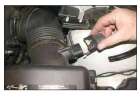
3. Squeeze the two locking tabs together, then remove the mass air electrical connection as shown.
