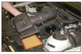
4. Loosen the hose clamp at the intake plenum and release the two clips that secure the air box lid to the vehicle. Remove the upper air box and intake tube as shown.
