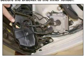
14. Re-install the head light module with the original hardware that was removed in step 5.NOTE: Install provided spacer under front mount as shown, then re-install module cover.
