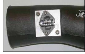
20. Secure the mass air sensor assembly into the K&N® intake tube with the provided hardware as shown
