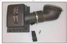
16. Remove the two screws that secure the mass air sensor to the air box with the provided Torx wrench, then remove the mass air sensor.
