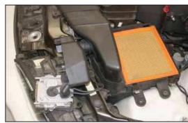
6. Lift the head light module and place out of the way on the core support to gain access to the lower air box for removal.
