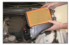
7. Remove the lower air box assembly as shown. NOTE: K&N Engineering, Inc., recommends that customers do not discard factory air intake.
