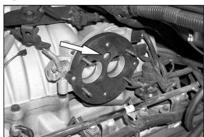
11. Install adapter base plate as shown.
