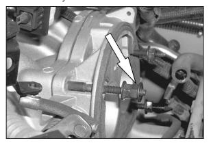
8. Using the stock nuts, create a jam nut on the stock stud and loosen the 4 studs.
