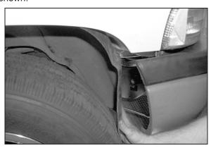
15b. Remove the 3 inner fender mounting retainers by pushing the center release pin in with an 1/8" punch.
