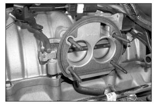
9. Remove throttle body gasket from throttle body.
