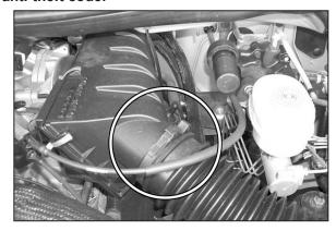
2. Remove plastic hose clamp at the air box as shown
