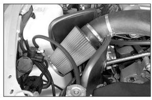
34. Install the K&N Air Filter onto the new K&N® intake tube as shown.
