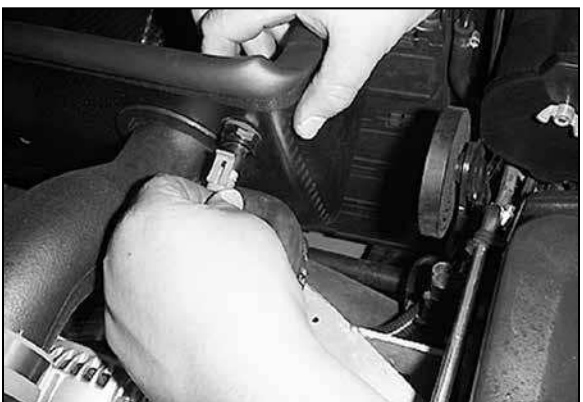
29. Reconnect the air temperature electrical connection.
