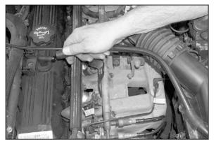
2. Disconnect the crank case vent hose.
