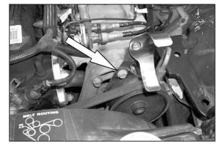
9. Using the bolt removed in step 7, secure the saddle bracket assembly to the upper power steering pivot as shown, but do not tighten completely at this time.
