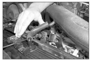
19. Install the 5 inch hose onto the crankcase vent, then connect the other end to the vent on the K&N^ $^{\mbox{\tiny (8)}}$  intake tube as shown
