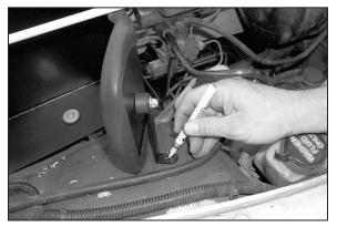
14. Install the bracket onto the K&N<sup>®</sup> heat shield and line up the bracket with the inner fender then mark the hole and drill a  $\frac{1}{4}$ " hole.
