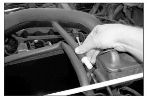
21. Connect the hose to the vent on the K&N<sup>®</sup> intake tube, then, connect the other end to the EVAP canister vent line as shown.
