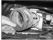
9. Loosen hose clamp that retains the rubber hose to the throttle body, then remove as shown.
