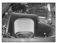
36. Install the K&N<sup>®</sup> air filter onto the K&N<sup>®</sup> intake tube as shown and secure with the hose clamp. NOTE: Drycharger<sup>®</sup> air filter wrap; part number RF-1034DK is available to purchase separately. To learn more about Drycharger<sup>®</sup> filter wraps or look up color availability please visit http://www.knfilters.com<sup>®</sup>.
