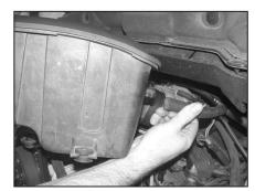
7. On 2007 and earlier model vehicles, disconnect the crankcase vent hose from resonator box as shown, then remove resonator box from vehicle
