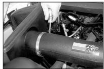
27. Using the provided hose clamp, secure the K&N<sup>®</sup> intake tube to the saddle bracket assembly as shown.
