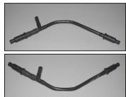
33. Rotate the long side of the vent tube assembly  $180^{\circ}$  as shown.
