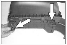
10. Remove the two rubber bushings from the factory airbox as shown.
