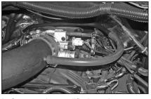
30. Connect the modified crankcase vent hose to the  $K\&N^{\circledast}$  intake tube as shown.
