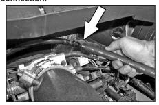
29. On models that the crankcase vent hose is connected to the "T" on the drivers side of the engine, remove the factory vent hose from the "T" fitting as shown.
