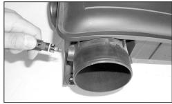
25. On models that come equipped with temp sensors, remove the air temp sensor from the resonator box as shown.
