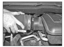
2. Loosen the hose clamp that connects the intake tube to the resonator box then remove the intake tube.
