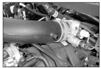
26. Install the intake tube onto the throttle body with the provided hose clamp.
