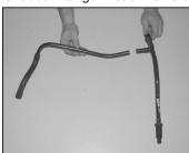
32. Cut the crankcase vent tube 1" from the "T" fitting as shown.
