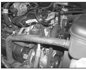
21. On 2007 and earlier model vehicles, install saddle bracket assembly onto engine using the provided hardware as shown.
