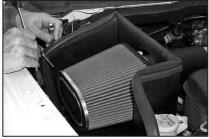
37. Align the heat shield for best clearance then tighten all the brackets.
