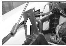
18. Remove the 8mm bolt that retains the airbox mount.
