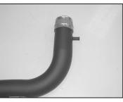
23. Install the provided silicone hose (08051) onto the K&N<sup>®</sup> intake tube with the provided hose clamp as shown.
