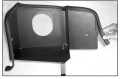
15. Install the provided edge trim onto the heat shield. Trim if necessary.
