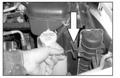
16. Remove the 13mm bolt from the upper fan shroud as shown.
