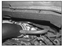
35. Connect the provided vent hose onto the "T" fitting,
