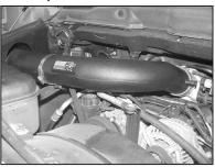
24. Install the intake tube onto the throttle body and saddle clamp and secure with the provided hose clamps as shown.
