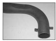
25e. Install the air temp sensor into the  $K\&N^{\ensuremath{\$}}$  intake tube as shown.
