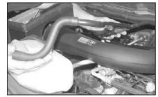
31. On models that the crankcase vent hose is connected to the "T" on the passengers side of the engine, remove the complete vent tube assembly from the rubber fittings in each valve cover as shown.
