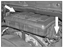
5. On 2007 and earlier model vehicles, remove the two 10mm bolts that retain the resonator box onto the engine
