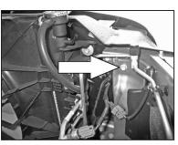
17. On 2009 and later model vehicles, remove the bolt shown from the radiator core support.
