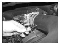
28. On models equipped with a air temp sensor, reconnect the electrical connection as shown. **NOTE: Due to manufacturing tolerances, it may be necessary to use the provided extension harness to connect the inlet air temperature sensor electrical connection.**
