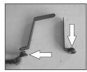
11. Install the two rubber bushings that were removed in the previous step into the provided brackets as shown.
