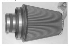
28. Install the silicone hose (08630) onto the K&N® air filter assembly and then secure with the provided hose clamp.
