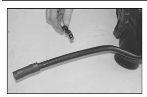
25. On 2005 and earlier vehicles remove the crankcase vent tube mounting clip from the crankcase vent tube on the airbox as shown.
