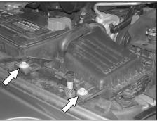
Remove the two airbox retaining bolts.
