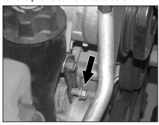
9. Remove the lower a/c bracket bolt shown with a 15mm socket.
