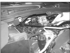
7a. On 2006 and later vehicles, disconnect the crankcase vent tube from the rear of the intake manifold.
