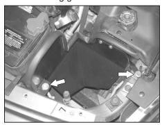
15. Install the K&N® heat shield assembly and secure the mounting bracket to the radiator core support with original bolt removed in step #13. Secure the rear of the heat shield to the 3/8" threaded insert with the provided hardware.
