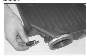
17. Twist the temp sensor counter clockwise to unlock and remove the temp sensor from the factory resonator.
