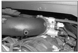
21. Install the intake tube onto the throttle body with the provided hose clamp.
