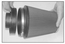
27. Install the provided radiused filter adapter into the K&N® air filter and secure with the provided hose clamp.
