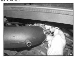
23. Reconnect the temp sensor electrical connection.
