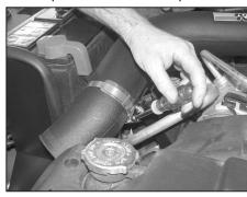
22. Using the provided hose clamp, secure the  $K\&N^{@}$  intake tube to the saddle bracket assembly as shown.
