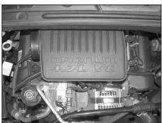
7. Remove the two 10mm resonator retaining bolts, then remove the resonator from the vehicle.
