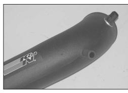
20. Install the air temp sensor into the  $K\&N^{\mbox{\scriptsize 6}}$  intake tube as shown.
