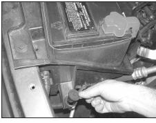
14. Install the 3/8" threaded insert provided into the airbox mounting grommet hole vacated in step #13.
