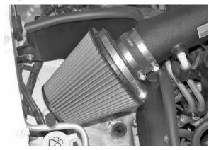
30. Install the air filter assembly onto the K&N® intake tube as shown and secure with the provided hose clamp.
