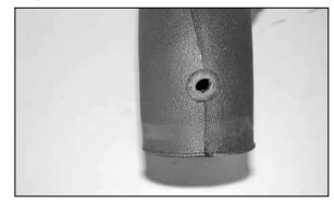
19. Install the provided grommet in the  $K\&N^{\otimes}$  intake tube as shown.
