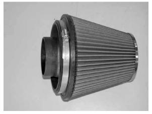
28. Install the filter adapter into the air filter as shown, secure with the provided hose clamp. NOTE: Drycharger® air filter wrap; part # RF-1048DK is available to purchase separately. To learn more about Drycharger® filter wraps or look up color availability please visit http://www.knfilters.com®.
