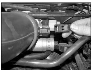
2. Release the locking tap on the air temperature sensor electrical connection, and then disconnect the electrical connection from the air temperature sensor.
