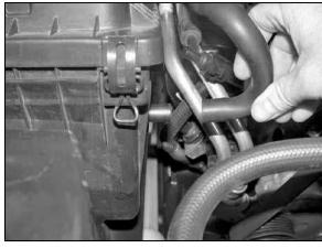
4. Disconnect the stock crankcase vent hose from the airbox as shown.
