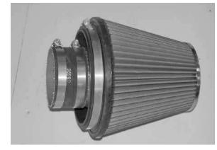
29. Install the silicone (08630) onto the air filter assembly and secure with the provided hose clamp.
