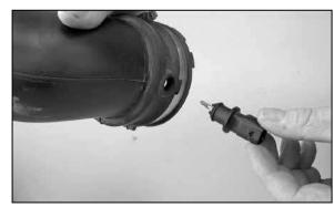
20. Remove the air temperature sensor from the stock intake tube as shown.
