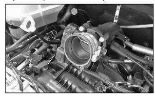
18a. On 2007 vehicles with a plastic throttle body, install the supplied silicone hose (084034) onto the throttle body and secure with the provided hose clamps as shown.
