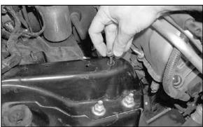
15. Vehicles that do not come equipped with cruise control, install the provided spacer and washer onto the stud as shown.
