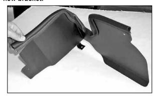
13. Install edge trim onto heat shield as shown. Trim if needed.
