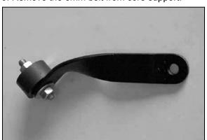
11. Assemble the bracket and rubber mounted stud as shown.
