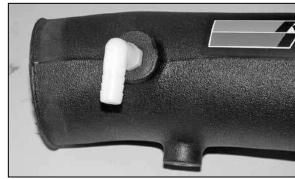
22. Install the 90° NPT fitting into the K&N $^{\! \rm 8}$  intake tube as shown.
