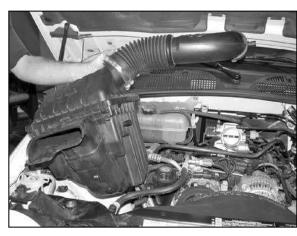
5. Firmly lift up to disengage the airbox from the retaining grommets and remove the airbox from the vehicle.
