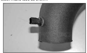
21. Install the air temperature sensor into the grommet in the K&N® intake tube as shown.
