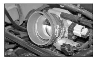
18. On 2006 and earlier vehicles, install the provided silicone hose (08690) onto the throttle body with the provided hose clamps as shown.
