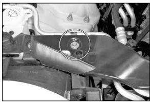
10. Remove the 6mm bolt from core support.
