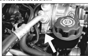
17. Remove the A/C compressor-mounting bolt.
