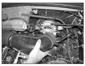
3. Loosen the hose clamp that secures the intake tube to the throttle body, and then disconnect the intake tube from the throttle body.
