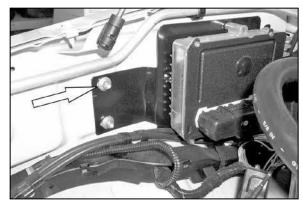
7. Remove nut from inner fender on vehicles that come equipped with a TCM.
