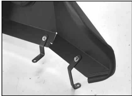
11. Install the “C” bracket (010118) onto the heat shield with the provided hardware as shown.
