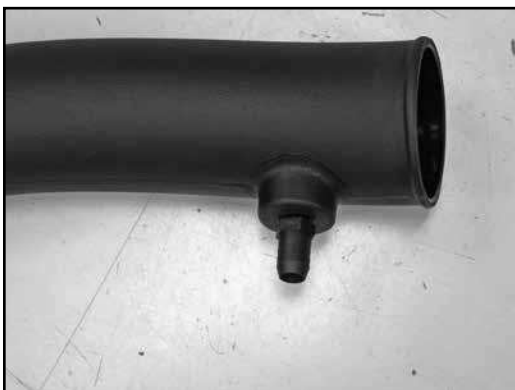
18. Install the provided 1/4”npt fitting into the K&N® intake tube as shown.
