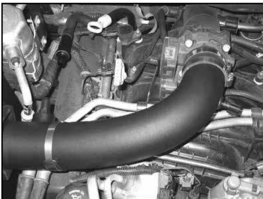
23. Install the K&N® intake tube into the into the silicone hose on the throttle body and position so the tube aligns with the saddle clamp. Secure the tube with the provided hose clamps.
