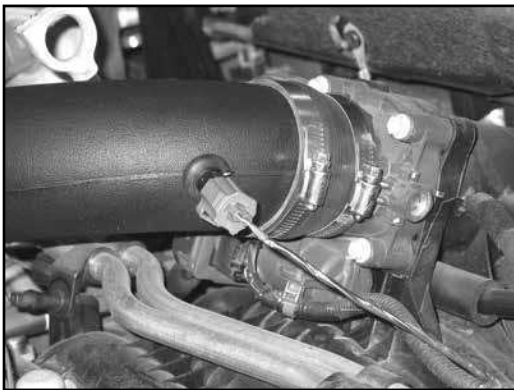
24. Reconnect the air temperature sensor electrical connection.
