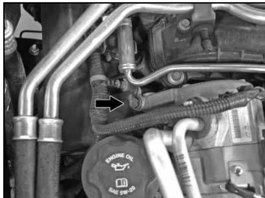
14. Remove the rear, lower A/C compressor mounting bolt shown.
