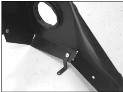
10. Install the “Z” bracket (010120) onto the heat shield with the provided hardware as shown.
