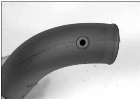
19. Install the provided grommet into the K&N® intake tube as shown.
