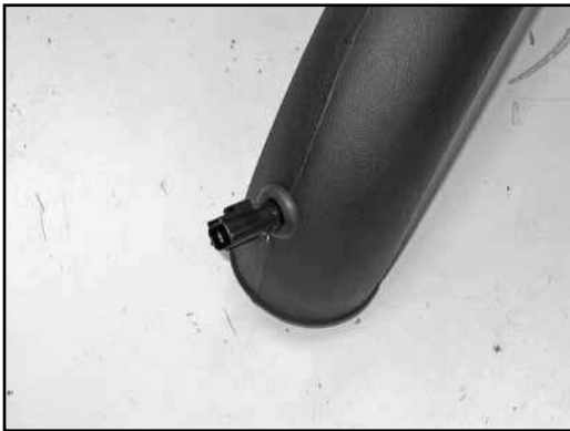
22. Install the air temperature sensor into the grommet installed into the K&N® intake tube in step #19.
