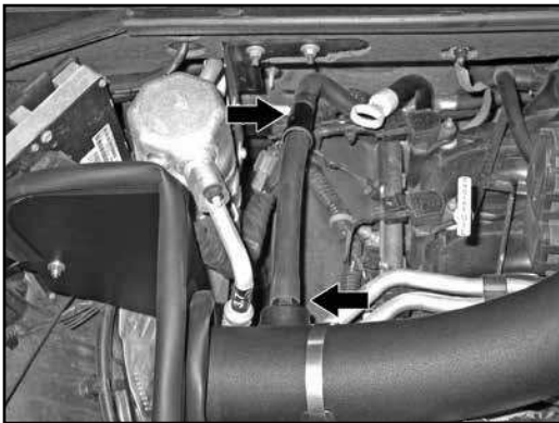
25. Install the provided silicone hose onto the 1/4npt fitting installed in the K&N® intake tube and then attach the open end onto the hose to the factory crank case tube.
