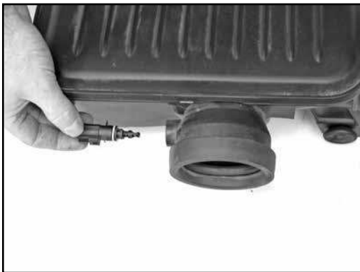
20. Twist the air temperature sensor counter clockwise and remove it from the stock intake plenum.
