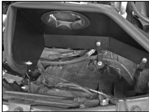
13. Install the heat shield assembly and secure with the provided hardware and the factory mounting nut. Be sure to remove the factory spacer on the air box mounting stud before installing the heat shield.
