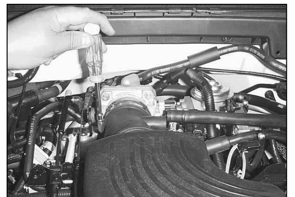
5. Loosen the hose clamp on the stock intake tube at the throttle body.
