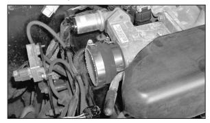
12. Install the provided silicone hose onto the throttle body with the provided hose clamps.
