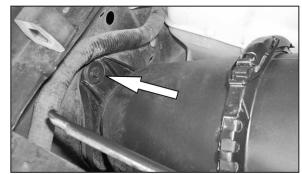
8. Release the push clip that secures the air box onto the vehicle.
