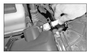
4. Disconnect the mass air electrical connection as shown.
