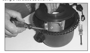
25. Using a flat blade screwdriver, push in and release the four clips that retain the mass air sensor retaining plate.
