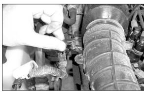
5. Disconnect the mass air wiring loom from the intake tube as shown.
