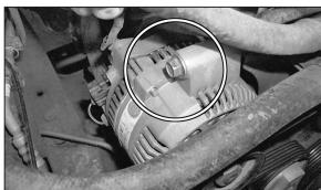
14. Remove the bolt that retains the alternator onto
