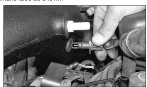
19. Install the air temp. sensor into the new K&N intake tube as shown.
