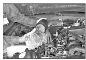
7. Remove the intake tube as shown.
