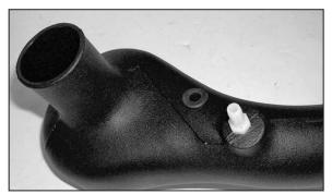
11. Install the vent fitting into the K&N intake tube as shown.
