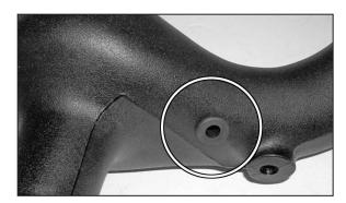
10. Install the provided grommet into the new K&N intake tube as shown.
