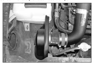
30. Install the mass air assembly onto the new intake tube then tighten the hose clamp.
