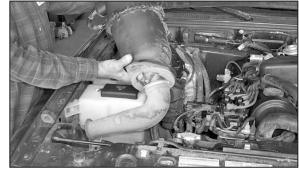
9. Pull firmly up on the air box to remove from vehicle.
