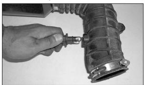
18. Remove the air temp. sensor from the stock intake tube as shown.
