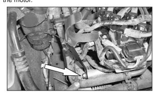
15. Install the saddle bracket assembly onto the alternator with the bolt that was removed in the previous step.
