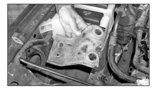
16. Remove the two bolts that retain the air box mounting bracket to the vehicle then remove bracket from vehicle.
