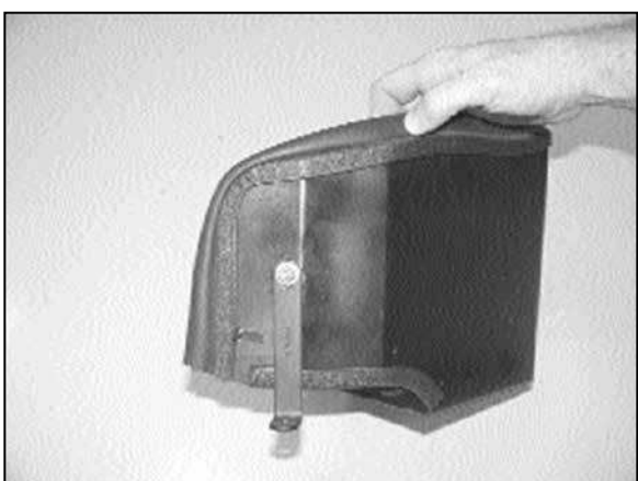
11. Install the "L" bracket onto heat shield as with the provided hardware as shown. NOTE: Install a washer between the bracket and heat shield.
