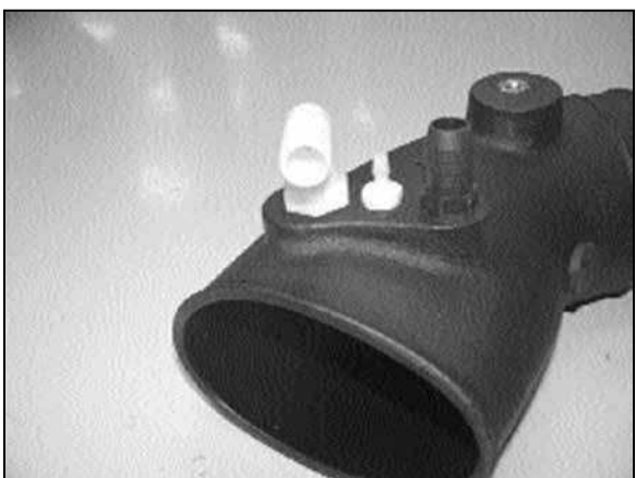
16. Install the provided vent fitting onto the new K&N intake tube as shown. NOTE: Plastic NPT fittings are easy to cross thread. Install the vent fitting "hand" tight, then turn it two complete turns with a wrench.
