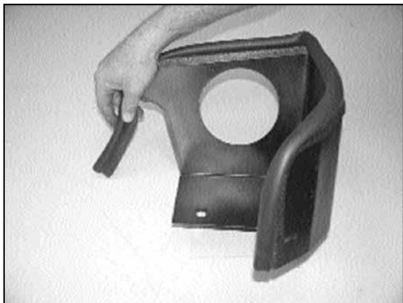
9. Install edge trim onto the heat shield as shown. Trim if needed.
