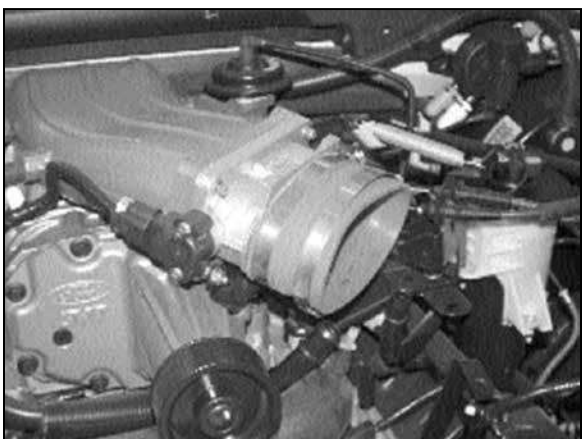
15. Install the silicone hose (08540) onto the throttle body with the provided hose clamp as shown.
