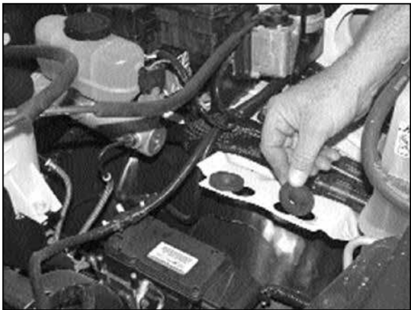
7. Remove the two air box mounting grommets from the air box mounting tray as shown.
