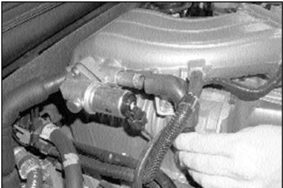
18. Remove the idle air vent tube from vehicle as shown.
