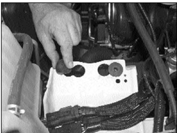
10. Install the two provided nut inserts onto the air box mounting tray as shown.
