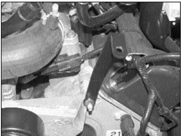
14. Install the provided bracket onto the stud with the nut that was removed in the previous step.
