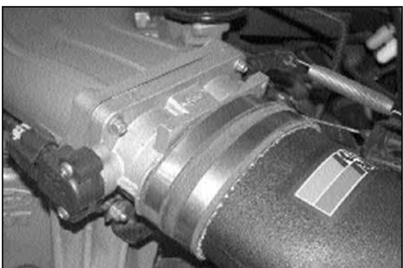
21. Install the new K&N intake tube into the silicone and then tighten the provided hose clamp. NOTE: Reconnect the three vent lines under the intake tube that were removed in step 4.
