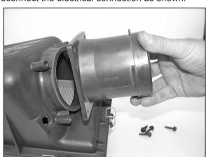
25. Remove the mass air sensor from the factory air box as shown.
