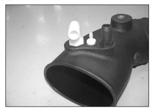
16. Install the provided vent fitting onto the new  $K\&N^{\tiny \circledR}$  intake tube as shown.
