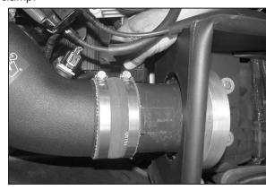
29. Reconnect the mass air sensor electrical connection as shown.
