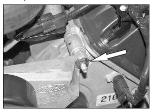
13. Remove the 8mm nut from stud that retains the idler pully bracket.
