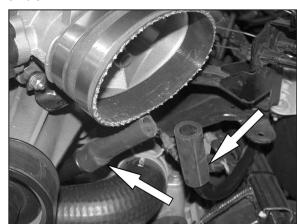
20. Install the two provide 5/8 silicone hoses onto the idle air and crank case vent lines as shown.
