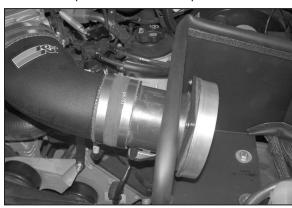
28. Install the mass air sensor assembly onto the intake tube, then secure with the provided hose
