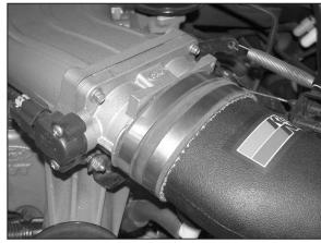
21. Install the new K&N® intake tube into the silicone and then tighten the provided hose clamp. NOTE: Reconnect the three vent lines under the intake tube that were removed in step 4.
