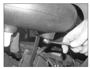
22. Connect the new intake tube to the bracket with the provided hardware as shown.
