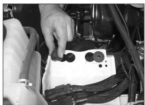
10. Install the two provided nut inserts onto the air box mounting tray as shown.
