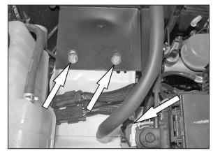
12. Install the heat shield into vehicle, then secure with the provided hardware as shown.
