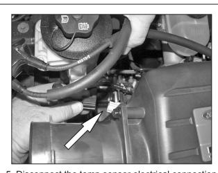
5. Disconnect the temp sensor electrical connection as shown.
