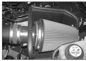
30. Install the Filtercharger onto the mass air adapter and then secure it with the provided hose
