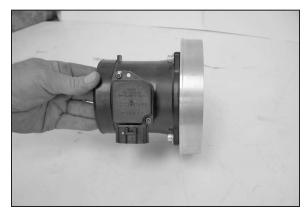
26. Assemble the filter adapter and gaskets onto the mass air sensor with the provided hardware as shown.
