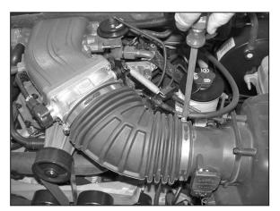
3. Loosen the hose clamp at the throttle body and mass air sensor as shown.
