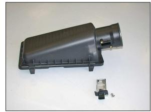
19. Using the "TORX" wrench provided, remove the mass air sensor from the air box lid as shown.
