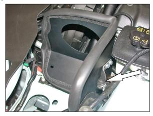
13. Install the heat shield into the vehicle and secure the bracket installed in step #12 to the factory air box mount with the factory bolt removed in step #9.
