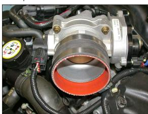
18. Install the provided silicone hose (08630) onto the throttle body and secure with the provided hose clamp
