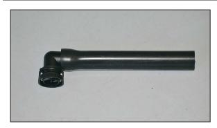
25. Install the provided 5/8" silicone hose onto the elbow removed in step #24 as shown.
