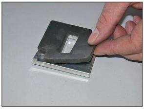
20. Install the provided gasket onto the K&N® mass air adapter as shown.
