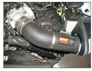
23. Install the K&N® intake tube assembly into the silicone hose at the throttle body and onto the saddle clamp and secure with the provided hose clamp as shown.
