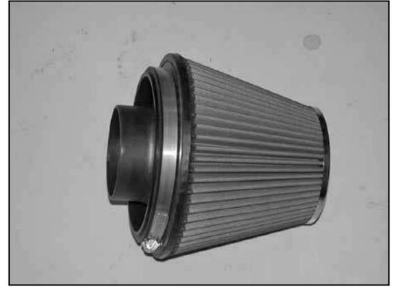
17. Install the filter adapter into filtercharger as shown and secure with the provided hose clamp.
