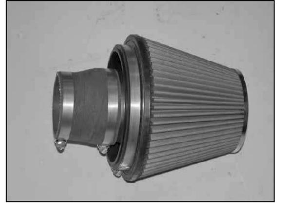
18. Install the silicone hose (08724) onto the filtercharger assembly and secure with the provided hose clamp as shown.
