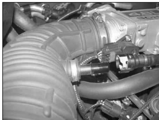
3. Release the green locking tab and then disconnect the crank case vent from the stock intake tube.
