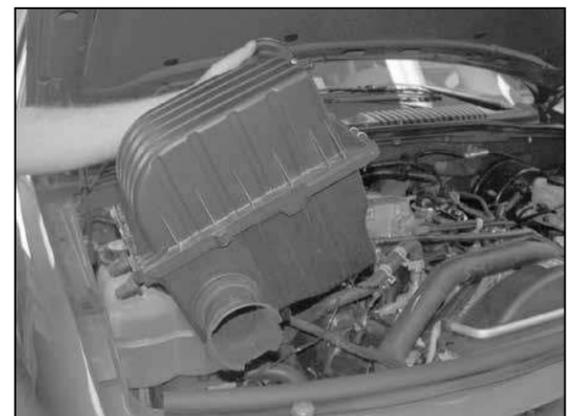
5. Using a screwdriver, pry up the bottom of the air cleaner to release the air cleaner from the mounting grommets, and then remove the air cleaner assembly as shown.
