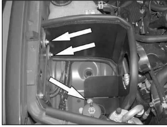
12. Install the heat shield as shown and attach to the inner fender with the factory coolant bottle mounting bolts and the 3/8" bolt and washer provided.
