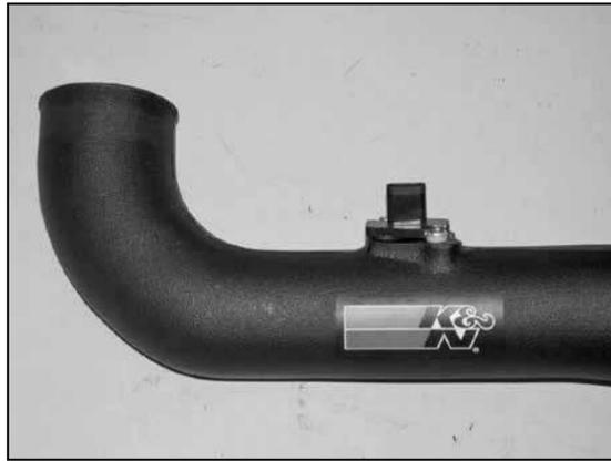
14. Install the mass air sensor into the K&N® intake tube and secure with the factory screws and spacers provided.
