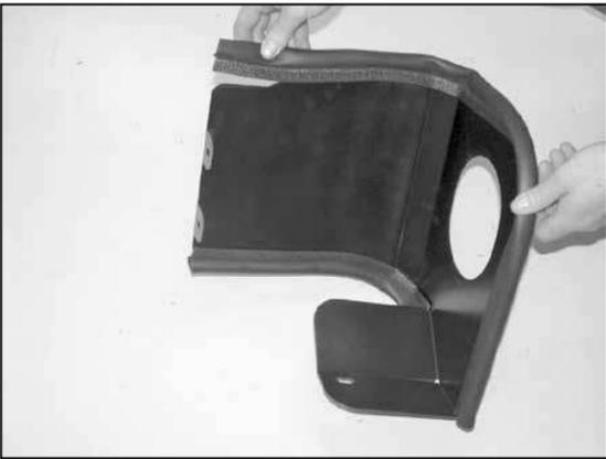
9. Install the edge trim seal onto the heat shield as shown.
