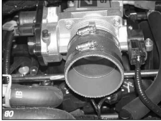
13. Install the silicone hose (08192) onto the throttle body and secure with the provided hose clamp as shown.
