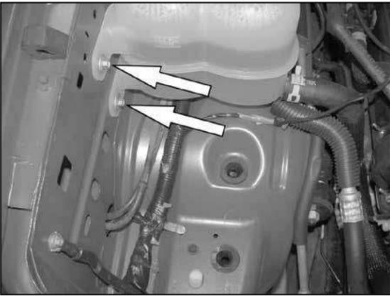
10. Remove the two-coolant bottle mounting bolts and the forward air box retaining grommet shown.
