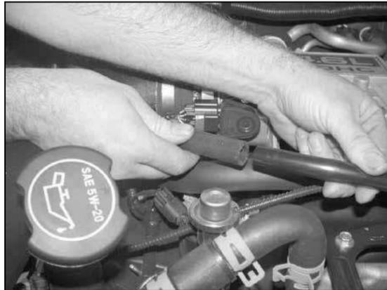
16. Cut the factory crank case vent tube one inch from the end, then attach the supplied silicone vent hose to the K&N® intake tube and factory vent tube as shown.
