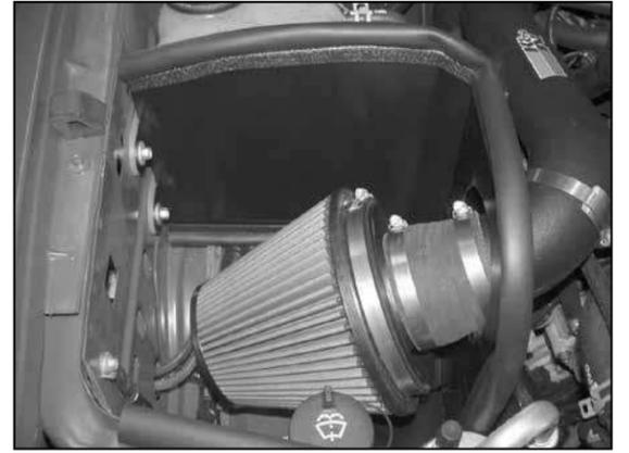
19. Install the filtercharger assembly onto the K&N® intake tube and secure with the provided hose clamp as shown.
