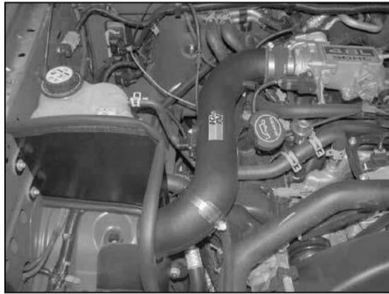
15. Install the K&N® intake into the silicone hose at the throttle body and onto the saddle clamp, then secure with the provided hose clamp.
