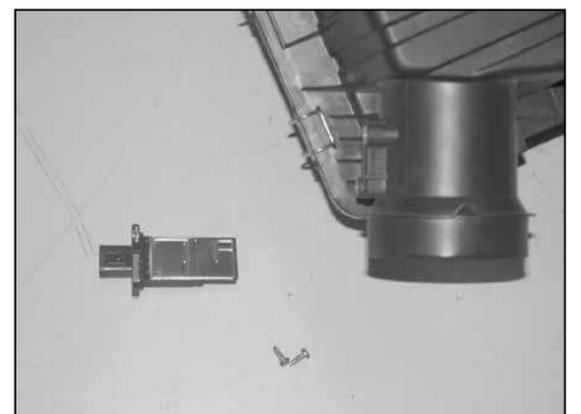
6. Using the "TORX" L key provided, remove the two screws, which retain the mass air sensor to the air box then remove the sensor as shown.
