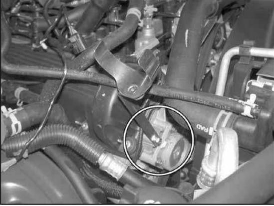
8. Using the 8mm bolt washers supplied, attach the tube mounting bracket assembly to the front of the engine at the threaded boss above the belt tensioner as shown.
