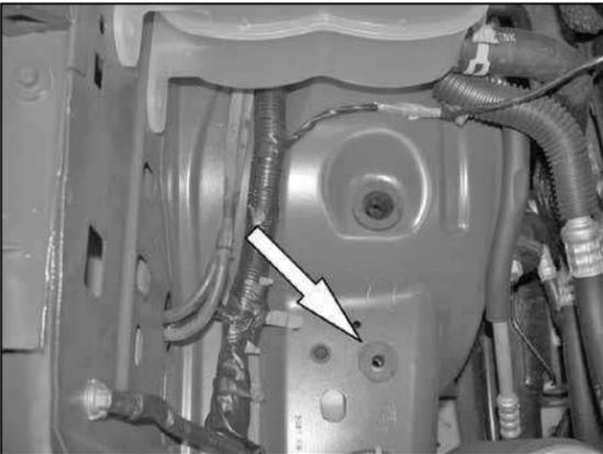
11. Install the inserted nut into the forward air box mounting grommet hole vacated in step #10 as shown.
