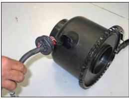
16. Slide the rubber grommet back to gain access to the mass air sensor electrical connector. Using a small screwdriver, release the red locking tab and disconnect the electrical connection, then remove the wiring harness.
