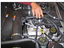
27. Install the supplied crank case vent hose onto the valve cover and secure with the provided hose clamp. Connect the other end onto the intake tube as shown.
