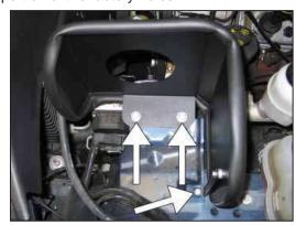
14. Secure the heat shield mounting bracket to the inner fender with the provided hardware and tighten the two inserted nuts.
