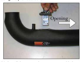
21. Install the mass air sensor assembly into the  $K\&N^{\circledcirc}$  intake tube and secure with the provided hardware.
