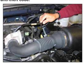
2. Rotate the crank case vent hose locking rings and pull the crank case vent hose off of the valve cover and intake tube as shown.
