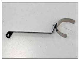
7. Install the saddle bracket onto the tube mounting bracket as shown.
