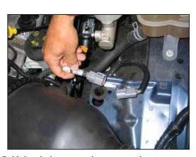
5. Unhook the secondary mass air sensor connection from the clip that secures it to the air box mounting bracket, then disconnect the secondary mass air connection.
