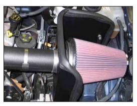
26. Install the filter assembly onto the intake tube and secure with the provided hose clamp.
