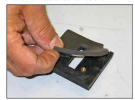
19. Install the supplied gasket onto the mass air sensor adapter as shown.
