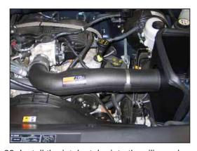
23. Install the intake tube into the silicone hose at the throttle body and align with the saddle clamp. Secure the intake tube with the provided hose clamp.
