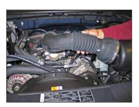
3. Loosen the hose clamps that secure the stock intake tube to the throttle body and air filter housing; remove the intake tube from the vehicle.
