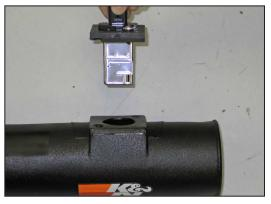
18. Install the mass air sensor assembly into the K&N<sup>®</sup> intake tube and secure with the provided hardware as shown.
