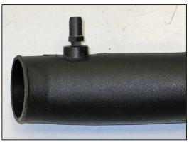
19. Install the  $1\!\!\!/4"$  NPT fitting into the K&N $^{\otimes}$  intake tube as shown.
