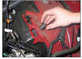
9. Remove the factory air box mounting grommets and replace them with the provided nut inserts as shown.
