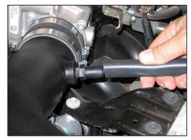
24. Connect the provided crank case vent hose onto the fitting on the valve cover and the vent fitting on the K&N<sup>®</sup> intake tube.
