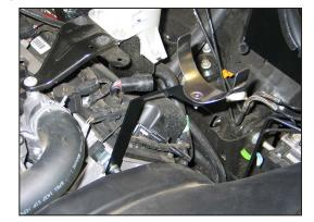
then seperate the mass air sensor housing from the factory air box.
