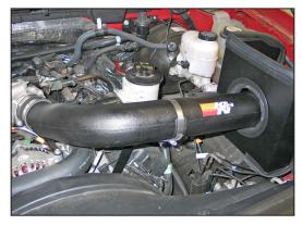
23. Install the K&N<sup>®</sup> intake tube into the silicone hose at the throttle body and align the intake tube with the saddle clamp. Secure the intake tube with the provided hose clamps.
