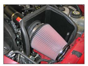
27. Install the air filter assembly onto the K&N<sup>®</sup> intake tube and secure with the provided hose clamp.
