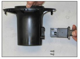
15. Remove the two mass air sensor retaining screws and remove the mass air sensor as shown.
