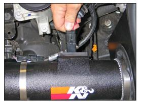
28. Re-attach the mass air sensor secondary connection to the power steering reservoir bracket, then connect the mass air sensor electrical connections as shown.
