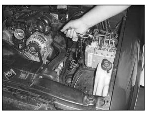
12. Using a 10mm socket, remove the bolt on the ABS bracket as shown above.
