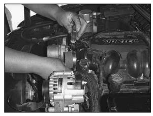
20. Install and secure the silicone hose onto the throttle body using the hose clamp provided as shown above.
