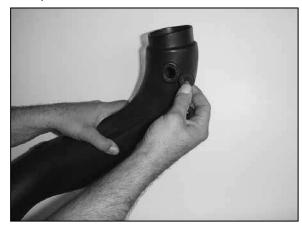
18. Install the two grommets provided into the  $K\&N^{\circledast}$  intake tube as shown above.
