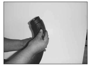
19. Remove the air temperature sensor from the factory intake hose and reinstall it into the grommet hole on the underside of the K&N<sup>®</sup> intake tube as shown above.
