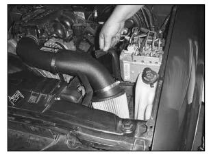
25. Install the trim seal provided onto the heat shield as shown above. NOTE: Some cutting and trimming will be necessary to achieve the best fit. 26. Reconnect the vehicle's negative battery cable. Double check to make sure everything is tight and properly positioned before starting the vehicle.
