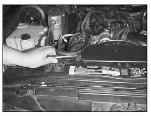
3. Using a flat blade screwdriver, release the push clip that secures the plastic resonator chamber to the radiator fan shroud.
