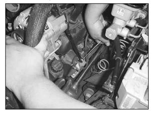
9. Reposition the stabilizing bracket, reinstall upper bolt and tighten both bolts.
