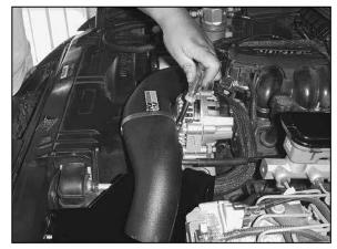
23. Install the hose clamp provided around intake tube and saddle and tighten as shown above.
