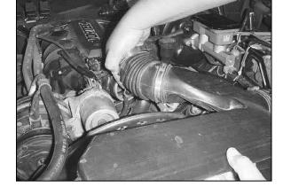
4. Remove the rubber intake hose from the throttle body and disconnect the air temperature electrical connection located on the underside of the rubber intake hose. 6. Remove the complete air intake assembly from the engine compartment. NOTE: K&N recommends that you do not discard factory air intake.
