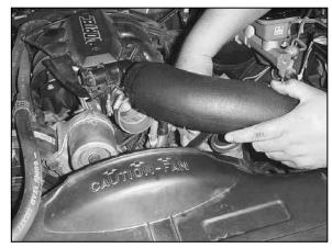
21. Install the K&N<sup>®</sup> intake tube, resting comfortably on the saddle/bracket and inserting the one end of the tube into the silicone hose. Reconnect the air temperature sensor electrical connection and insert the vent hose into the grommet hole located on the backside of the K&N tube.
