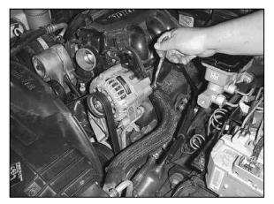
7. Loosen and remove the top on the alternator stabilizing bracket. Loosen the lower bolt and swing bracket out of the way.
