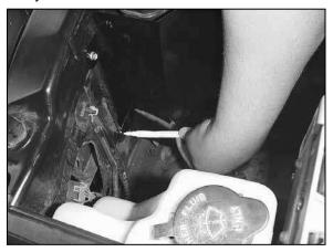
14. Install the self tapping screw into the existing hole in the radiator core support. Mark the lower hole of the heat shield when it lines up with the radiator core, fully exposing the factory opening in the core support.
