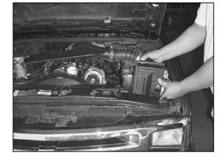
2. Loosen the hose clamp located on the rubber intake hose at the throttle body.
