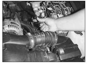
5. Remove the vent hose from the factory intake tube.
