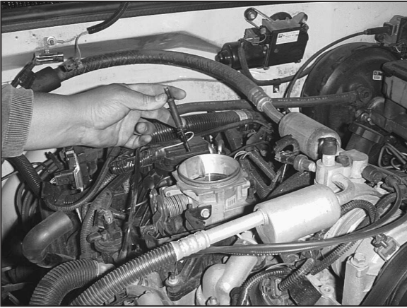
10. Using a 7/32" socket, loosen and remove the factory stud off from the throttle body.
