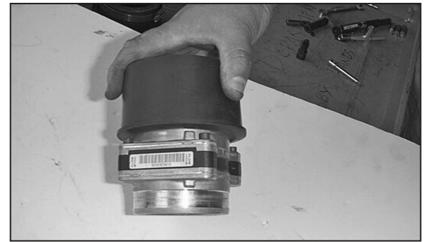
21. Install the filter adapter onto the mass air sensor with the directional arrow as shown above.
