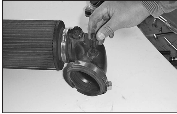
13. Remove the air temperature sensor from the factory intake tube.
