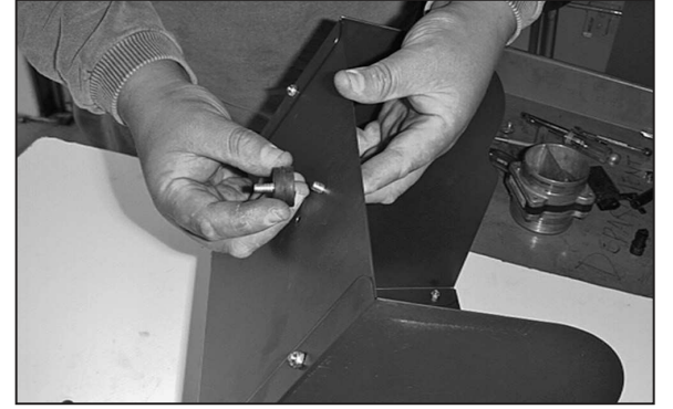
20. Using the provided hardware, install the rubber mounted studs onto the bottom side of the heat shield.
