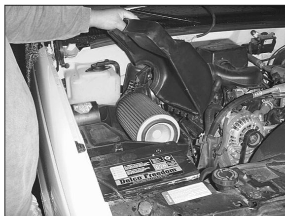
3. Release the over center clamps and remove the the airbox lid.
