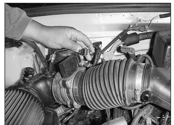
6. Disconnect the mass air sensor electrical connection.
