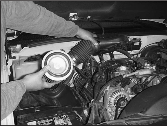
7. Lift and remove the complete air intake system.
