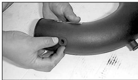
27. Install the 1" OD grommet into the hole in the primary intake tube.
