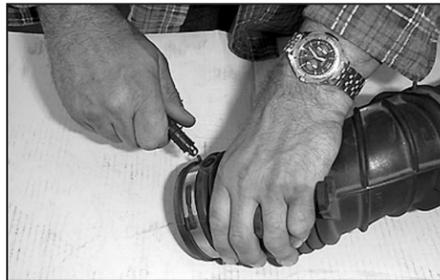
26. Remove the air temp. sensor from the stock intake tube and air box top.
