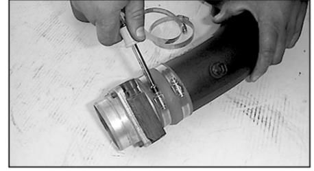
30. Using the hose clamp provided, attach the silicone step hose to the mass air sensor with the directional arrow as shown above.
