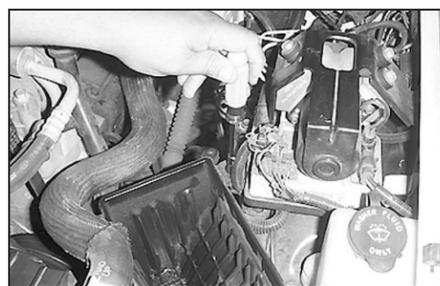
7. Loosen and remove the bolt that retains the air box base.
