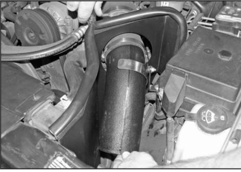
38. Install the secondary intake tube into the silicone hose and secure with provided hose clamp.
