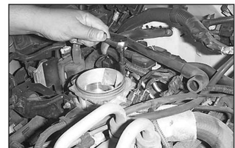
10. Using a 7/32" socket, loosen and remove the factory stand off from the throttle body.
