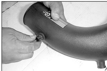
28. Install the air temp. sensor into the grommet.
