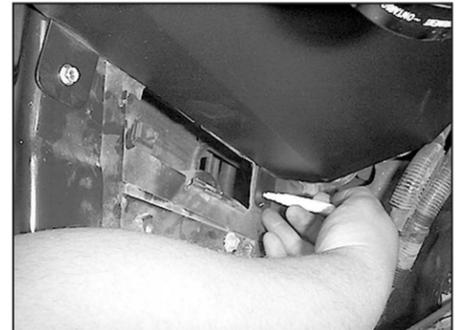
33. Mark the lower hole on the heat shield.
