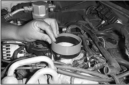
19. Install the 4" ID silicone hose over the adapter and tighten using a provided midi clamp.
