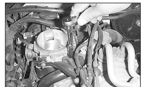
12. Remove the nut that retains the throttle cable bracket.
