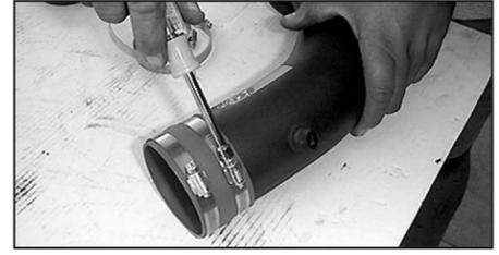
29. Using the hose clamp provided, attach the silicone step hose onto the end of the primary intake tube.
