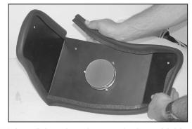
11. Install the edge trim onto the heat shield. NOTE: Some trimming of the edge trim may be necessary.
