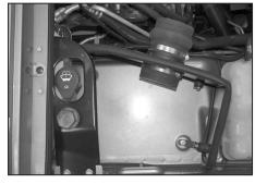
19. Secure the brackets to the heat shield with the provided hardware. Do not tighten completely.
