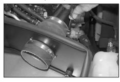
21. Install the intake tube onto the vehicle; then align the tube with the mass air sensor and then tighten hose clamp.
