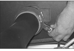
24. Reconnect the mass air electrical connection as shown.
