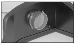
17. Install the silicone hose (08621) on the inside of heat shield with the provided hose clamps.
