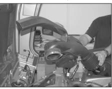
6. Detach the intake tube from the throttle body and mass air sensor then remove the intake assembly.
