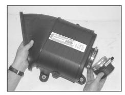
9. Loosen the hose clamp that retains the mass air sensor onto the air box then remove the mass air sensor from the air box.
