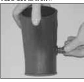
32. Install the air temp sensor into the primary intake tube as shown.
