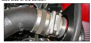
28. Install the mass air sensor assembly onto the K&N® intake tube and secure with the provided hose clamp.
