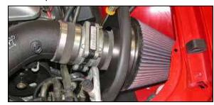
29. Install the air filter assembly onto the K&N® intake tube and secure with the provided hose clamp.
