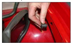
24. Install the threaded insert into inner fender as shown.
