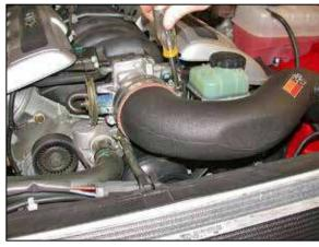
17. Install the K&N® intake tube onto the throttle body as shown and secure with the provided hose clamp, using the 8mm bolt provided. Secure the K&N® intake tube onto the mounting bracket installed in step #12.
