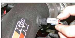
31. Reconnect the temperature sensor electrical connection.
