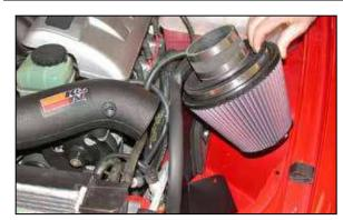
22. Set the heatshield assembly onto the inner fender, then set the air filter assembly between the heatshield and fender as shown.
