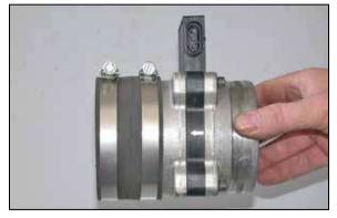
27. Install the silicone hose (#08630) onto the intake tube side of the mass air sensor and secure with the provided hose clamp.
