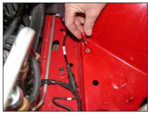
11. Remove the inner airbox mounting stud shown with a T-30 torx socket.
