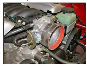
13. Install the silicone (08755) onto the throttle body and secure with the provided hose clamp.
