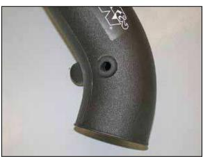
15. Install the provided rubber grommet into the K&N® intake tube as shown.
