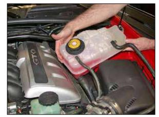
7. Pull the coolant reservoir up and away from the inner fender to release it from the retaining studs.
