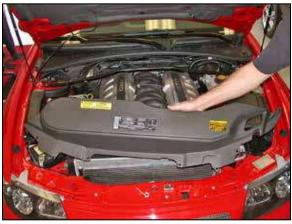
3. Lift up on the radiator cover and pull back to release from the retaining hook, then remove the cover from the vehicle.
