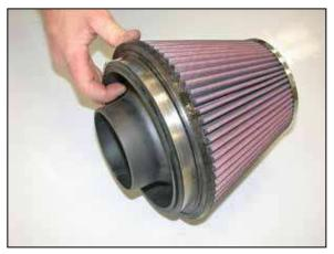
19. Install the radiused filter adapter into the K&N® air filter as shown. Secure with the provided hose clamp.
