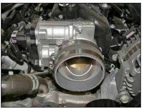
17. Install the provided silicone hose (08625) onto the throttle body and secure with the provided hose clamp as shown.
