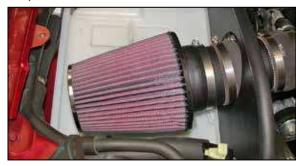
23. Install the K&N® air filter onto K&N® intake tube and secure with the provided hose clamp. NOTE: Drycharger® air filter wrap; part # RF-1032DK is available to purchase separately. To learn more about Drycharger® filter wraps or look up color availability please visit http://www.knfilters.com®.
