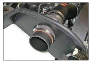
22. Install the "EH" tube assembly onto the mass air sensor and secure with the provided hose clamp.
