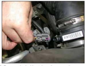
2. Depress the locking tab on the mass air sensor electrical connection and then separate the connector from the mass air sensor.
