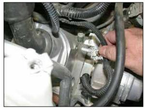
11. Unthread the retaining clip from the engine as shown.
