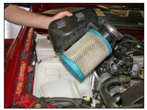
8. Remove the stock air filter assembly from the vehicle as shown.
