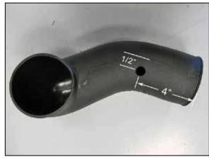
18a. On vehicles equipped with a crank case vent, mark the tube 4" back from the end of the tube and  $\frac{1}{2}$ " below the mold seam then drill a 5/8"id hole.
