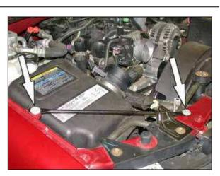
4. Remove the two bolts, which secure the core support brace to the core support and inner fender, and then remove the brace from the vehicle.
