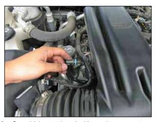
hose, unhook the crank case vent from the intake tube as shown.
