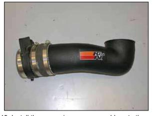
19. Install the mass air sensor assembly onto the K&N intake tube (EI) as shown.
