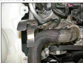
13. Install the tube bracket assembly onto the engine using the hardware provided.
