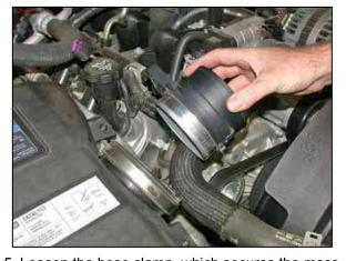
5. Loosen the hose clamp, which secures the mass air sensor to the air box, then remove the mass air sensor from the air box.
