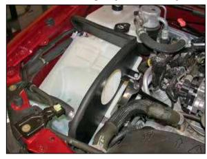
16. Install the heat shield assembly into the vehicle using the provided hardware.
