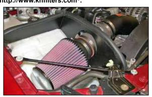
24. Re-install the core support brace removed in step #4 with the stock hardware.
