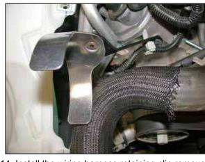
14. Install the wiring harness retaining clip removed in step #11 into the new tube mounting bracket, and then rescuer the wire harness to the clip as shown.
