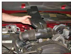
3. Loosen the two hose clamps which secure the stock intake tube, mass air sensor and throttle body, then lift the intake tube to release it from the rubber mount on the intake manifold and remove it from the vehicle.
