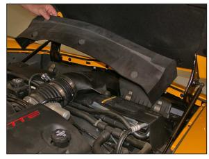
2. Unsnap the ends and then remove the air filter
