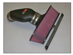
10. Install the filter-mounting bracket onto the air filter as shown and secure with the provided hardware.
