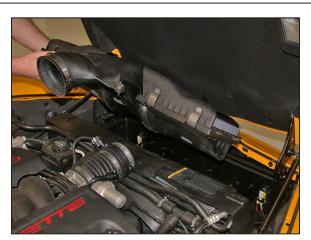
4. Pull up on the complete intake system to disconnect it from the air box mounting pins and then remove it from the vehicle as shown. **NOTE: K&N Engineering, Inc., recommends that customers do not discard factory air intake.**
