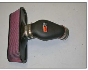
9. Install the silicone hose (08536) onto the K&N<sup>®</sup> intake tube and secure with the provided hose clamps.
