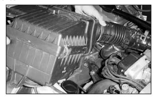
6. Detach the intake tube from the throttle body, pull upward firmly on the airbox to release it from it's retaining grommet and remove the entire air intake assembly.
