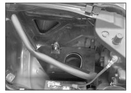
15. Install the heat shield assembly into the vehicle as shown. Secure the rear heat shield mounting bracket to the fresh air duct with the bolt removed in step #11. Secure the forward heat shield mounting bracket to the inner fender with the provided hardware as shown.
