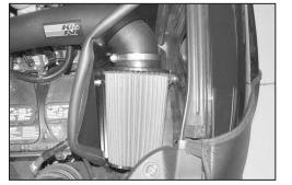
21. Install the air filter onto the K&N<sup>®</sup> intake tube and secure with the provided hose clamp.
