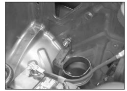
11. Remove the fresh air duct retaining bolt shown. **NOTE: This bolt will be reused.**
