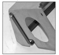
13. Install the provided "L" bracket #070026 onto the heat shield with the provided hardware as shown.
