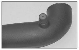
18. Install the provided rubber mounted stud onto the K&N $^{\circ}$  intake tube as shown.
