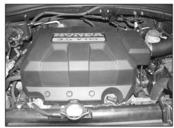
24. Reinstall the engine cover and secure in place with the three 1/4 turn fasterners.
