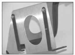
14. Install the provided "L" bracket #010054 onto the heat shield with the provided hardware as shown.
