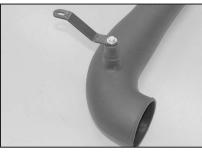
19. Install the tube mount bracket # 070065 onto the K&N^ ${\ensuremath{\mathbb S}}$  intake tube as shown.
