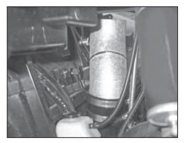
25. Install the K&N<sup>®</sup> intake tube into the silicone hose and align with the tube mounting bracket installed onto the heat shield, then secure the intake tube with the hose clamp and hardware provided.
