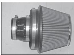
23. Install the silicone hose (08724) onto the filter adapter and secure with the provided hose clamp.
