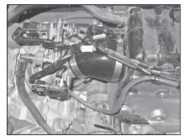
9. Reconnect the fuel injection electrical connections.
