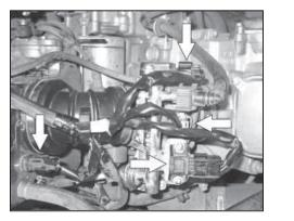
4. Unhook the four fuel injection electrical connections shown and place the wiring harness to the
