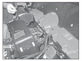
13. Remove the deflector shield as shown.
