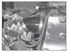
8. Install the silicone hose assembly onto the throttle body and air chamber and secure with the hose clamps.
