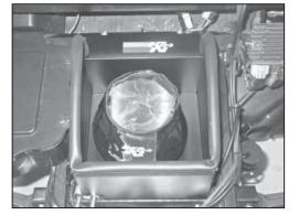
26. Install the K&N<sup>®</sup> air filter assembly onto the intake tube and secure with provided hose clamp.
