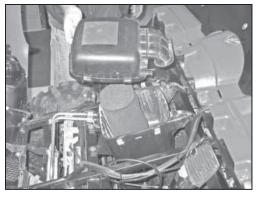
14. Unclip the five air box lid clips and remove the air box lid from the air box base.
