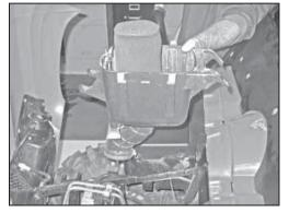
17. Remove the lower air box from the vehicle as shown.
