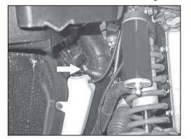
16. Loosen the hose clamp which secures the intake tube to the lower air box.
