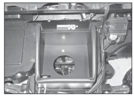
21. Install the heat shield assembly into the vehicle and secure with the provided hardware to the factory air box mounting locations.
