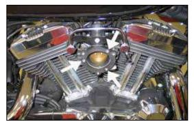
8. Install the K&N® intake tube adapter onto the throttle body using the provided hardware.
