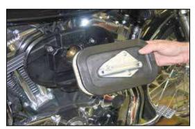
4. Remove the air filter as shown.
