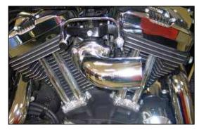
10. Install the K&N® intake tube onto the throttle body while attaching the vent hose to the vent tube and secure with the provided hardware.
