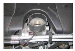
20. Install the provided silicone hose (08698) onto the throttle body and secure with the provided hose clamp.
