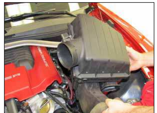
6. Remove the air box from the vehicle. NOTE: K&N Engineering, Inc., recommends that customers do not discard factory air intake.
