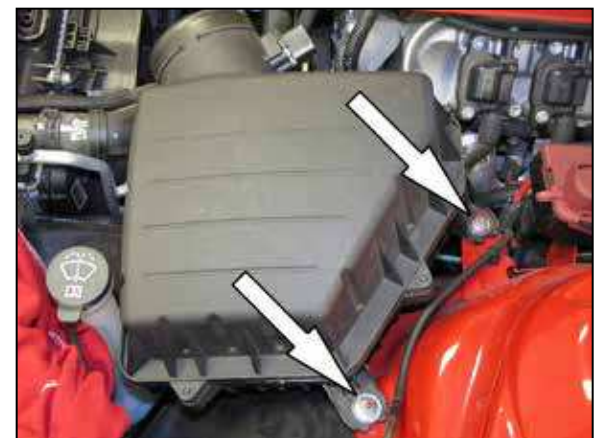
5. Remove the two air box mounting nuts shown.
