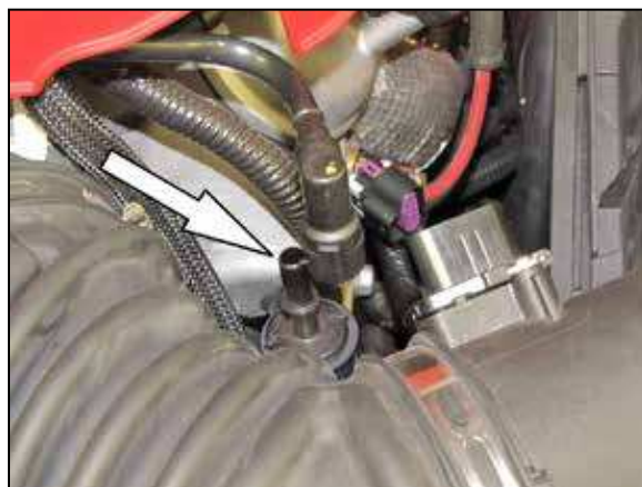
3. Disconnect the crank case vent from the intake tube.
