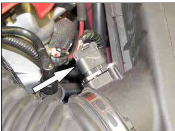
2. Disconnect the mass air sensor electrical connection.
