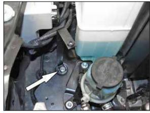
17. Install the provided secondary air pump mounting bracket (083169) onto the inner fender using the provided hardware.
