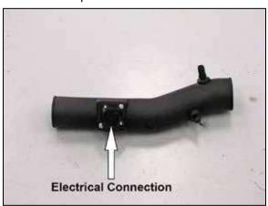
29. Install the mass air sensor assembly into the K&N® intake tube and secure with the provided hardware.
