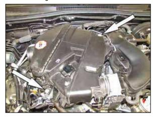
10. Remove the two bolts securing the air filter housing to the engine and then remove the air filter housing from the engine.
