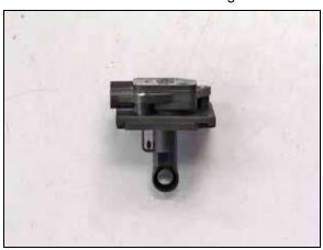
28. Install the mass air sensor into the adapter and secure with the provided hardware.
