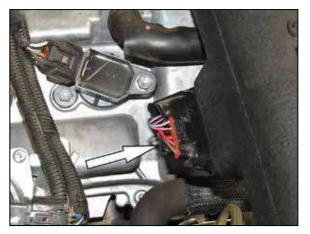
33. Reconnect the mass air sensor electrical connection.
