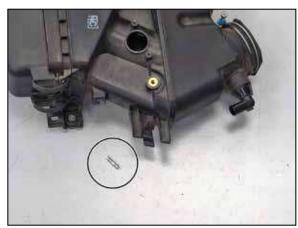
34. Remove the engine cover mounting stud from the factory air filter housing.
