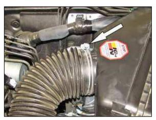
5. Loosen the hose clamp securing the intake tube to air filter housing.
