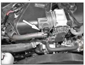
8. Release the spring clamp securing the crank case vent hose and then disconnect the crank case vent hose.
