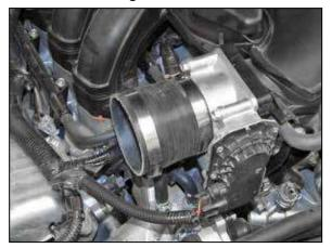
23. Install the provided silicone hose (08429) onto the throttle body and secure with the provided hose clamp.
