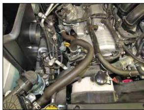
21. Install the secondary air pump onto the brackets previously installed and secure with the provided hardware. Reconnect the secondary air hose to the fitting and secure with the factory spring clamp.
