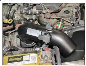
24. Install the K&N® intake tube assembly into the silicone hose at the turbo inlet and align with the mounting bracket installed on the heat shield. Secure the heat shield with the provided hardware and hose clamp
