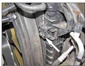
16. Remove the fan shroud bolt shown.
