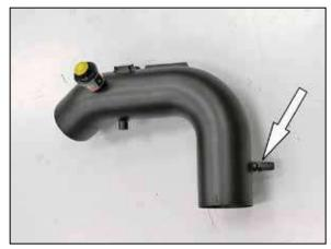
22. Install the 5/8 barb, 1/4npt crank case vent fitting provided into the K&N® intake tube as shown.
