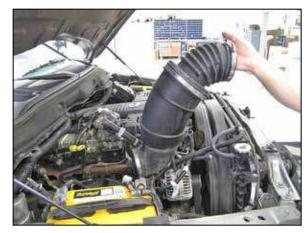
7. Loosen the hose clamp securing the factory intake hose to the turbo inlet and then disconnect the crank case vent hose from the pipe. Remove the complete intake hose from the vehicle as shown.
