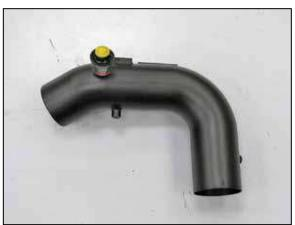
21. On vehicles equipped with a filter minder, install the factory grommet and filter minder into the  $K\&N^{\otimes}$  intake tube as shown.
