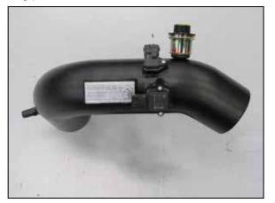
23. Install the inlet air temperature and mass air sensors into the K&N® intake tube using the
