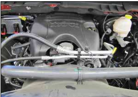
11. Reinstall the engine cover and route the crank case vent hose through the factory opening.
