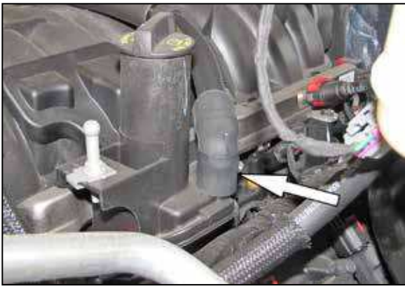
7. Disconnect the crank case vent hose assembly from the valve cover port.
