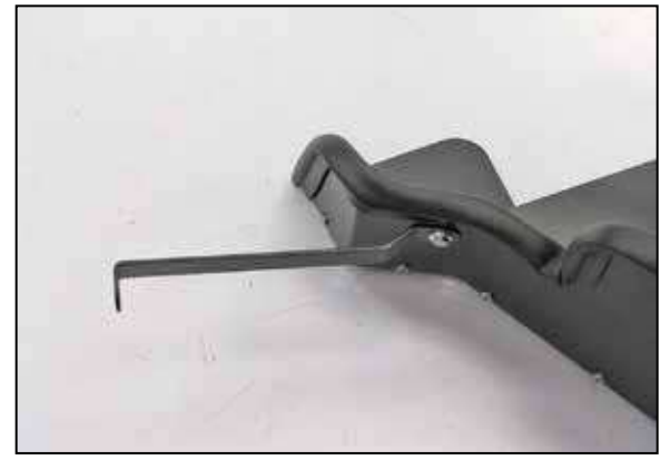
18. Install the provided mounting bracket (083103-1) onto the heat shield using the provided hardware.
