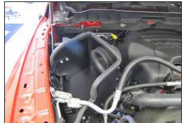
21. Install the heat shield into the vehicle and secure with the factory bolts from steps #19 and #20. NOTE: Do not completely tighten at this time.
