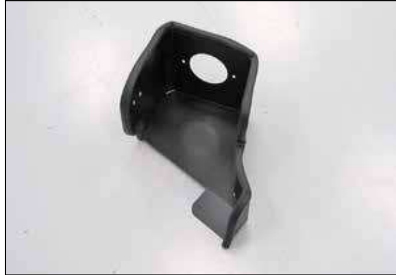
14. Install the provided edge trim onto the heat shield as shown. NOTE: Some trimming of the edge trim will be necessary.
