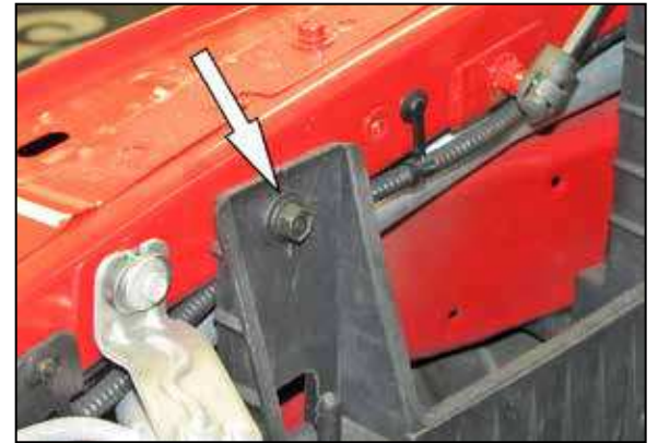
19. Remove the front air box mounting bracket bolt shown. NOTE: This bolt will be reused in a latter step.
