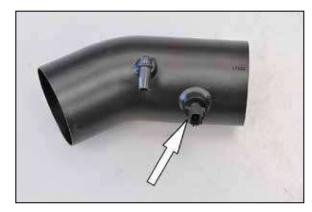
17. Install the inlet air temperature sensor into the  $K\&N^{@}$  intake tube as shown.
