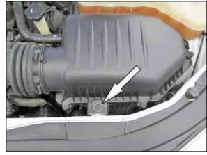
6. Remove the bolt which secures the air box to the core support.
