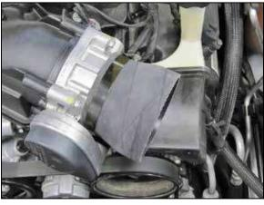
14. Install the silicone step hose (08050) onto the throttle body and secure with the provided hose clamp.
