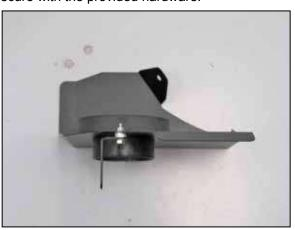
9. Install the provided heat shield mounting bracket (070742) along with the spacer onto the heat shield as shown.
