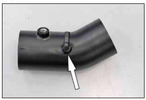
15. Install the provided 90° vent fitting into the K&N® intake tube as shown.
