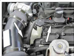
21. Install the assembled vent hose onto the fitting installed in the K&N® intake tube and then attach the open end to the valve cover port.
