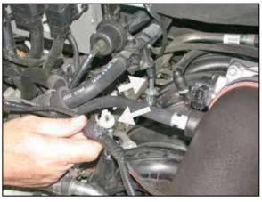
21. Reattach the heater hose and wiring harness to the studs installed in the previous step.
