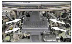
6. Remove the four bolts securing the air filter housing to the intake manifold.
