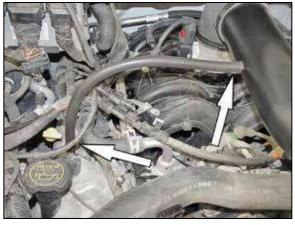
22. Install the provided crank case vent hose onto the vent port on the K&N<sup>®</sup> intake tube and then onto the vent on the valve cover.
