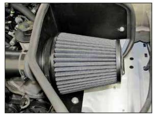
23. Install the K&N $^{\circ}$  air filter onto the filter adapter
