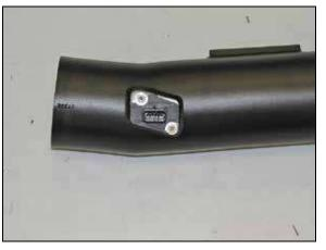
19. Install the mass air sensor into the  $K\&N^{\otimes}$  intake tube and secure with the provided hardware.
