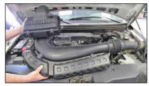
7. Remove the complete air box and intake snorkel assembly as shown.
