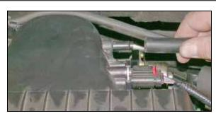
4. On vehicles equipped with a Brake Booster/ EVAP vent line, disconnect the vent line from the air box.
