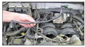
9. Release the crank case vent hose from the valve cover port and then remove the crank case hose from the vehicle.
