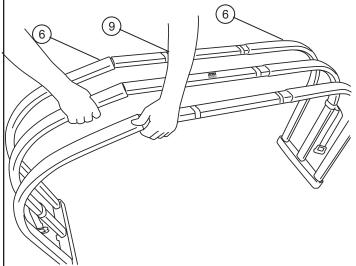
Slide 3 center tubes into the open ends of the bent tubes as shown. Insert center tube with logo into the center tube.
