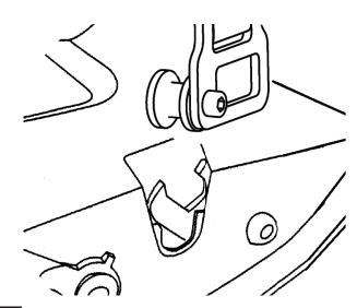
When the BEDXTENDER is at the furthest rear position, push down on the buckle to insert into tailgate latch. Tighten straps. To release, pull tailgate handle.
