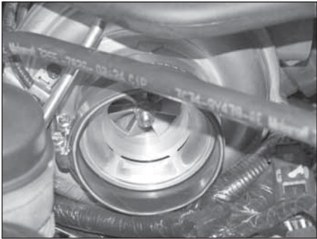
9d. On 2006 and later vehicles, install the silicone hose (08761) onto the turbo inlet and secure with the provided hose clamp.
