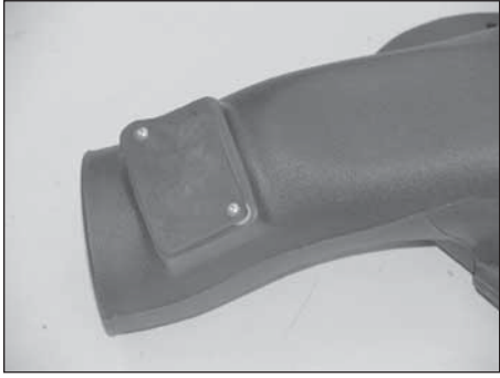
15. On vehicles equipped with an air temperature sensor, install the mass air block off plate onto the K&N® intake tube using the provided screws and spacers as shown.
