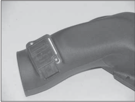
18. On vehicles equipped with the mass air sensor install the mass air sensor onto the K&N® air box lid with the provided screws and spacers as shown.
