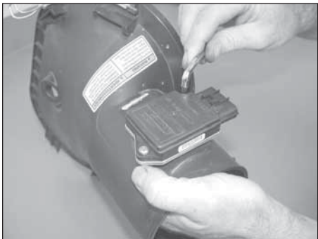
10. On vehicles equipped with a mass air sensor remove the mass air sensor from the factory air box lid with the provided torx wrench as shown.
