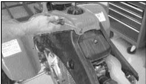
3. Remove all of the clips and fasteners from the front body shell and remove plastic side panels.
