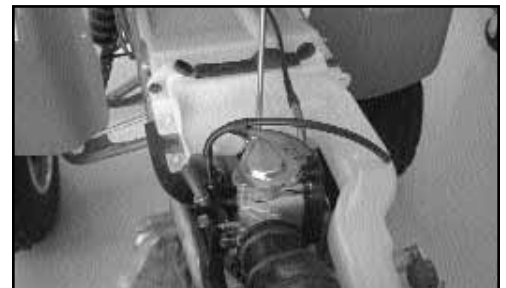
13. Remove the three screws from the needle slide cover located on the top of the carburetor. Remove the needle slide cover.
