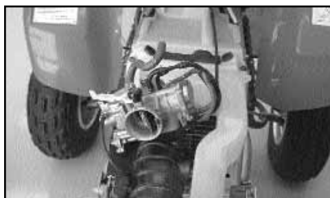
9. Remove the carburetor. Position the carburetor on top of the ATV for access to the float bowl and vacuum slide assembly.
