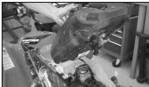
5. Remove all of the fasteners and straps from the fuel tank. Remove the fuel tank.
