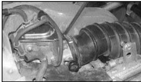
7. Loosen the hose clamp from the intake tube to the carburetor.
