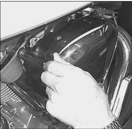
2. Remove the three air cleaner housing mounting bolts (two on top of the assembly and one on the bottom).
