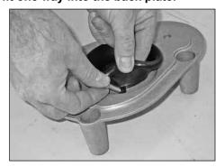
7. Install the three backing plate mounting bolts through the velocity stack.
