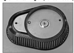
11. Install the cover stand-off onto the K&N® air filter as shown using the provided bolt.
