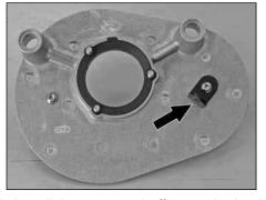
8. Install the two stand-offs onto the backing plate using the two provided bolts (07706). On models equipped with an intake valve solenoid pigtail, be sure to install the provided bracket with the bottom stand-off bolt.
