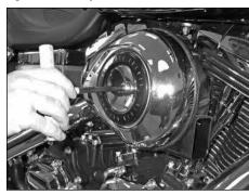
2. Remove the air filter cover mounting bolt and then remove the cover from the vehicle.
