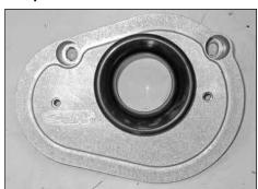
6. Install the provided venturi into the K&N® back plate as shown.
