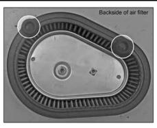
12. Make note of the breather ports on the backside of the air filter.
