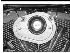
10. Install the backing plate onto the throttle body and secure with the bolts installed during step #7. Then secure the backing plate to the engine with the factory breather bolts.
