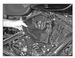
5. Remove the stock air filter base and gasket from the vehicle.
