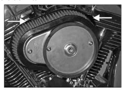
12a. Install the filter assembly onto the back plate as shown using the bolts provided. Be sure to apply Loctite onto the mounting bolts.
