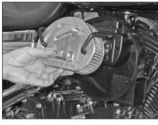
3. Remove the three air filter mounting bolts, unhook the two breather tubes from the breathers and then remove the air filter from the vehicle as shown. **NOTE: It will be necessary to remove the clip nut to access the lower mounting bolt.**
