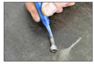
7. Apply one drop of the provided thread locker to the provided throttle body bolts.
