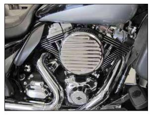
13. Install the K&N® air filter and front plate onto the back plate and secure with the provided hardware. NOTE: It may be helpful to use a small screwdriver to position the filter into the grooves of the front and back plate while tightening the hardware.
