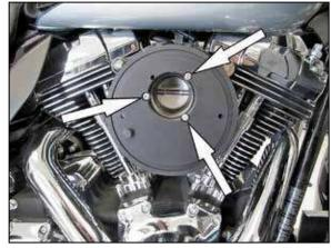
11. Install the filter back plate and gasket onto the adapter and secure with the provided bolts.
