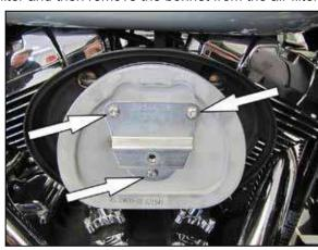
3. Remove the three bolts securing the air filter, then disconnect the crank case breather hoses and remove the air filter.
