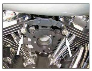
6. Install the K&N® adapter onto the engine and throttle body using the provided breather bolt. NOTE: Do not completely tighten the breather bolts at this time. Take care while installing the adapter so that the "O" rings do not get pinched.
