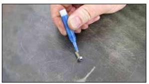
10. Apply one drop of the provided thread locker to the provided filter back plate mounting bolts.
