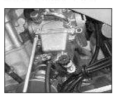
Loosen the four screws on the float bowl. NOTE: The float bowl may still contain fuel.
