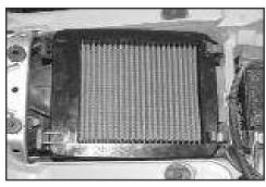
10. Install X-STREAM<sup>™</sup> POWERLID TM C onto the air box using stock retaining clips. NOTE: X-STREAM<sup>™</sup> POWERLID<sup>™</sup> will only fit in one direction.
