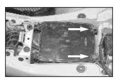
2. Unclip the two airbox retaining clips on lid and remove it.
