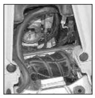
3. Loosen the clamp on the intake boot that runs from the air box to the carburetor then move aside.
