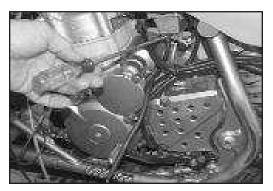
5. Locate the float bowl drain screw per ATV owners manual and drain the fuel from the
