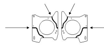
Trim the area as indicated by the arrows. Re-install the assembly behind radiator support. Only 2 of the 4 bolts will be used to re-install each headlight assembly. Depending on the year of the vehicle, the top mounting holes may need to be drilled.
