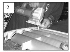
**Along the bottom**; make your cut about 1/16" to 1/8" inside the chrome ring. Taper the cut on each end into the cut along the bottom
