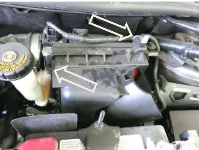
c. Unlatch the two clips holding the two halves of the air box together and remove the front section and air box by tilting it towards the front of the car and lifting it up and out.
