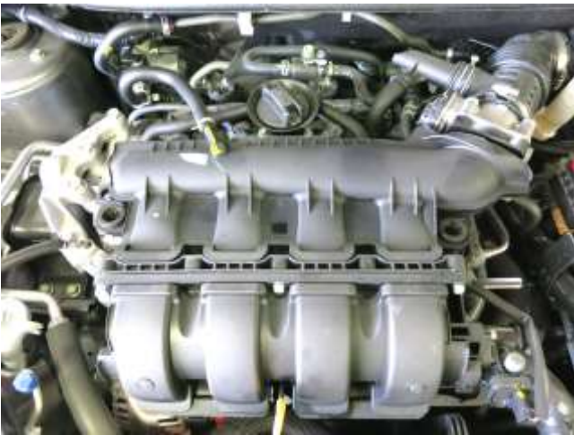
a. Remove plastic engine cover by pulling up with both hands gently.
