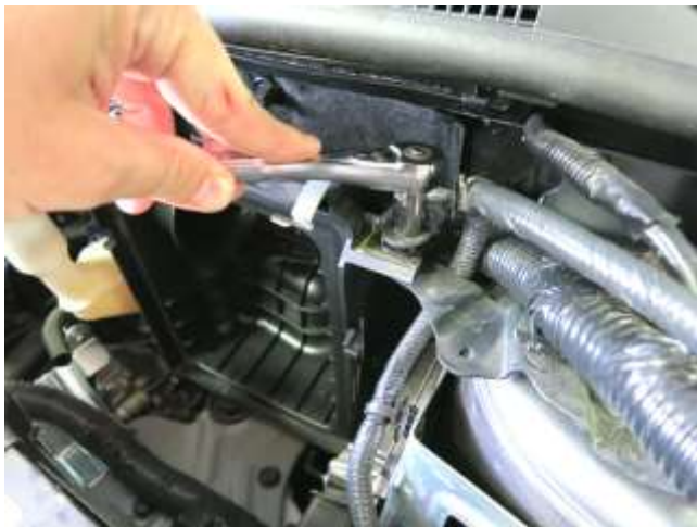
d. Unbolt the other section of the air box as shown.
