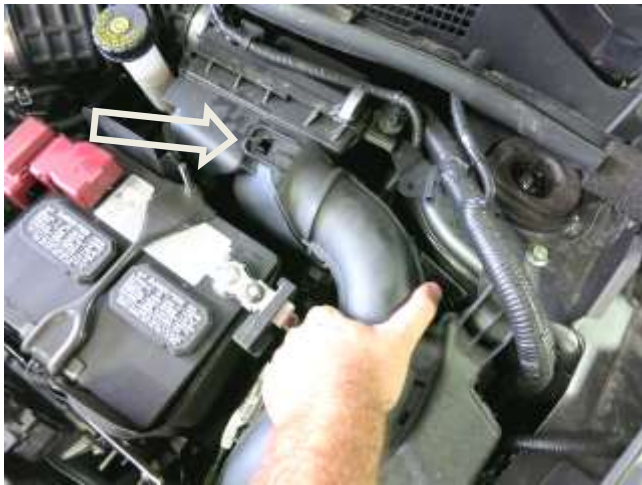
b. Remove the plastic air duct from the stock air box by pulling it straight up while lifting the tab where the arrow is pointing.
