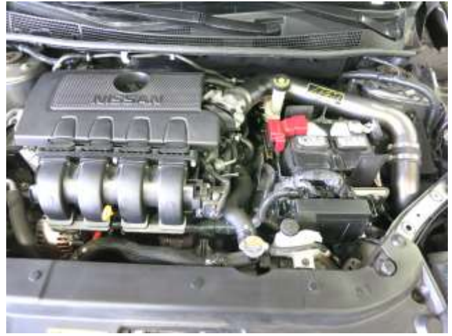
AEM INTAKE INSTALLED
