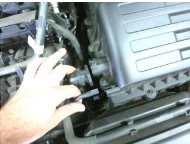
c. Remove small vacuum line from the stock air box. Remove the large air injection hose by depressing the ribbed parts of the collar. Note: Not all models will have this large hose.
