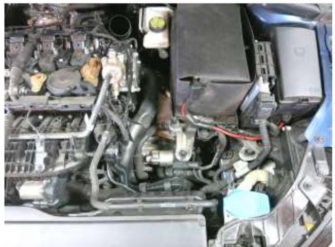
d. Remove the stock air box and intake hose assembly from the vehicle by pulling upwards to disengage the three rubber grommets. Lift the hose side first and maneuver the box towards the rear, clearing the cold air inlet.
