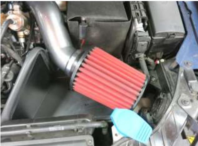
g. Install the AEM Dry Flow filter and hose clamp onto the intake tube and tighten to 30 in-lb. Position the tube for best fit and tighten the coupler and mounting bracket at this time.
