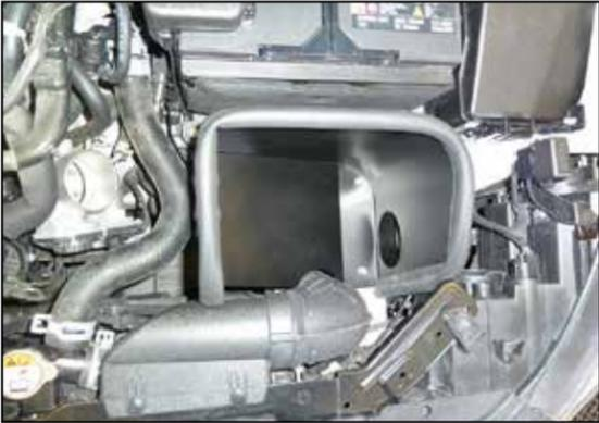
9. Install the heat shield into the vehicle so the studs protrude through holes in the heat shield, secure the heat shield with the provided hardware.
