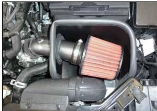
13. Install the air filter onto the intake tube, adjust the tube and filter for best fit and then secure with the provided hose clamps.
